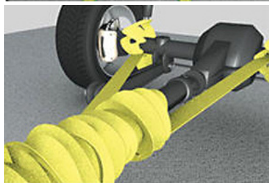
Tighten: The tendrils tighten the attached fabric straps around the drive shaft and axles, locking them in place to bring the car to an immediate stop
