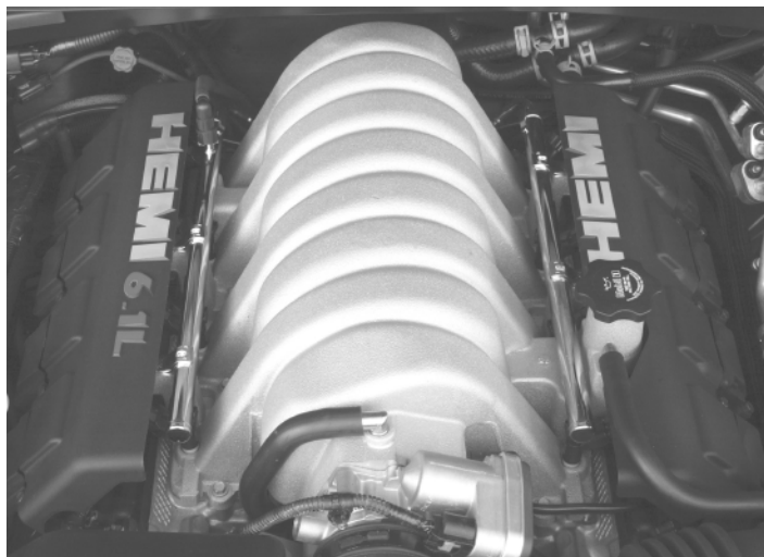
Chrysler Hemi 6.1-liter 425-horsepower engine.
